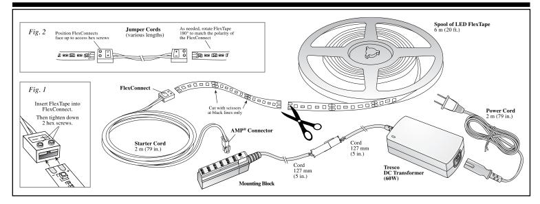
Tresco International's LED FlexTape light system is designed to adhere to a smooth, clean surface (indoor locations only). To be used with Tresco DC Transformer (60W) only.
