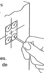
**H.** Drill a 1/2" (13mm) diameter hole 1-1/4" deep at each center point marked. Chisel away any excess wood required to allow strike box to seat in jamb.
