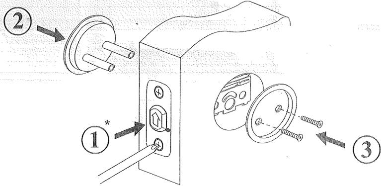
\*Proper installation allows the "thumb pull" to open from bottom, as shown.
