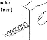
**F.** Trace face of latch in door edge and chisel out area 5/32" (4mm) deep.
