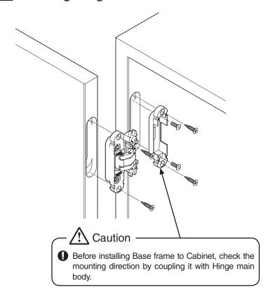
While holding the door, insert Hinge main body into the Base frame on Side board. Keep holding the door and fix the hinge with the fixing screws at once.
