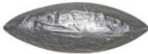
SATIN STAINLESS a hand-applied satin finish on warm, hand cast stainless steel
