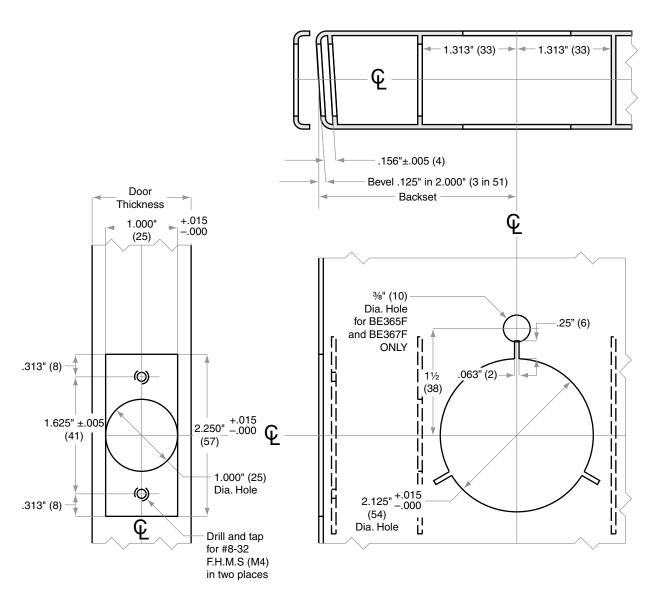
Dimensions shown in parentheses () are in millimeters.
