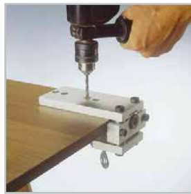
Drill the adjustment hole. Max opening of 1-3/4"
