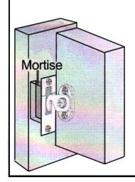
Turn lock latch to horizontal position. Level top of lock latch with stamped line on the strike plate. Mark and mortise jamb to accomodate lock latch and strike plate.
