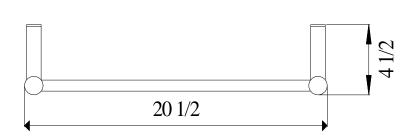
For construction with wall studs on 16 in. centers, the header is located between the studs for the right side mounting. For construction with wall studs on centers greater than 19-1/2 in. provide secure header as shown.
