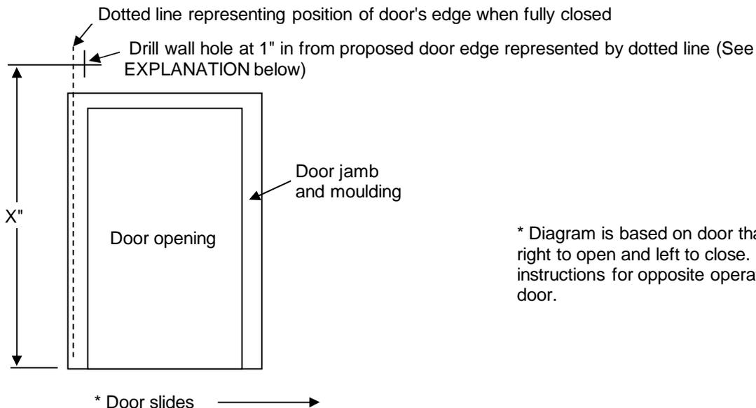
EXPLANATION - FOR HORIZONTAL LOCATION OF TRACK: Most doors can be mounted so the vertical edge of the door will be even with the extreme vertical edge of the track, when the door is in the fully closed position. Since the first hole is normally 1" from the track ends, simply calculate your horizontal track measurement 1" inward from where YOU WANT the edge of the door to be when in the fully closed position.
